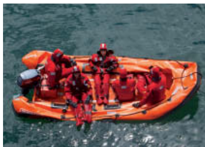
Insubmersible: Even with all its compartments deflated, the boat conserves its buoyancy with crew and equipment.
